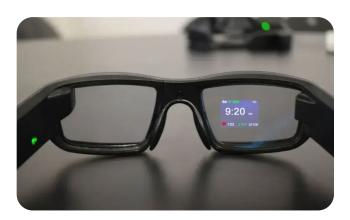
The HARVi Smart Glasses is one of the first all self-contained augmented reality smart glasses available. The see-through Waveguide optics merge digital instructions onto real-world tasks, removing distractions, vision occlusion and thereby reducing error rates.
