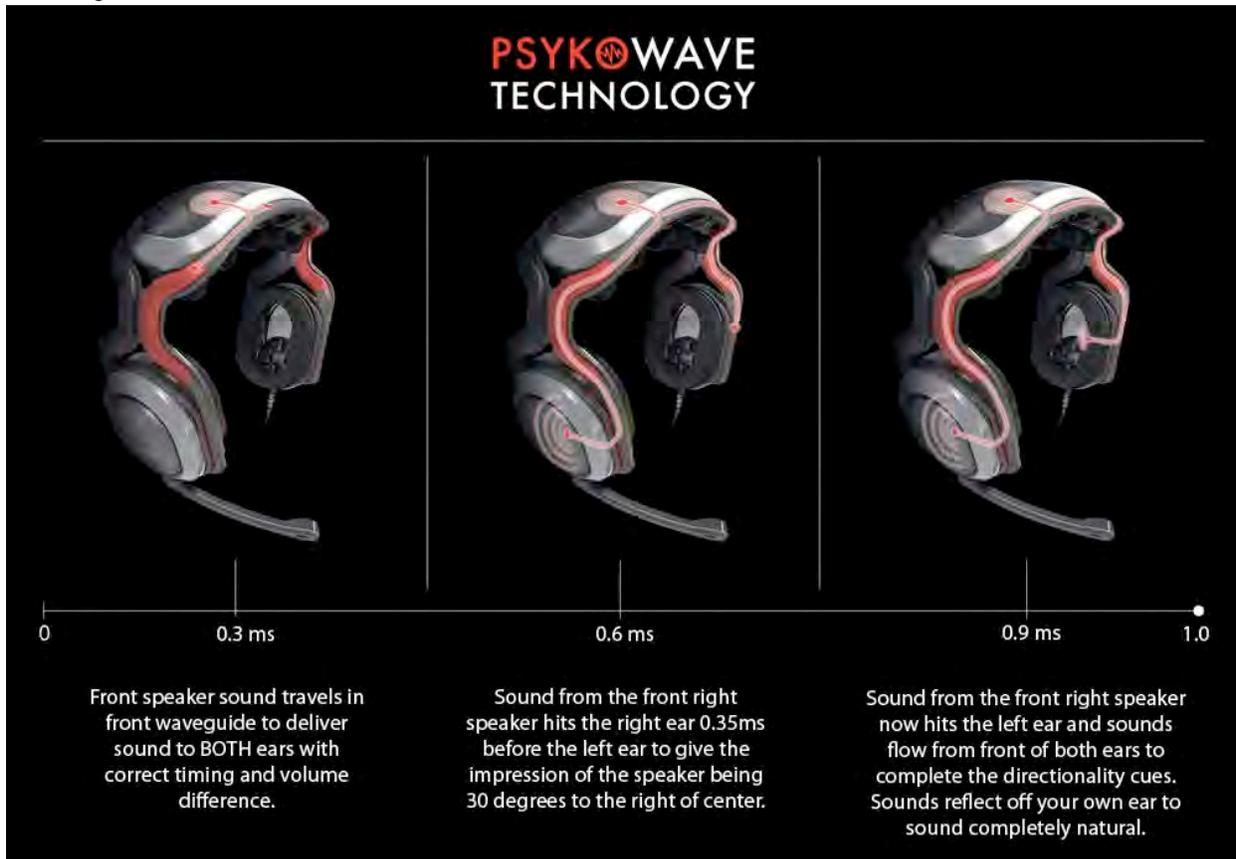
Unlike the virtual methods, the Psykowave technology has no latency, a pinna effect unique to each person and the transition from one position to another requires no interpolation functions. In fact the Psykowave technology is exactly like a room speaker system, where the sound moves completely smoothly from one position to another.
